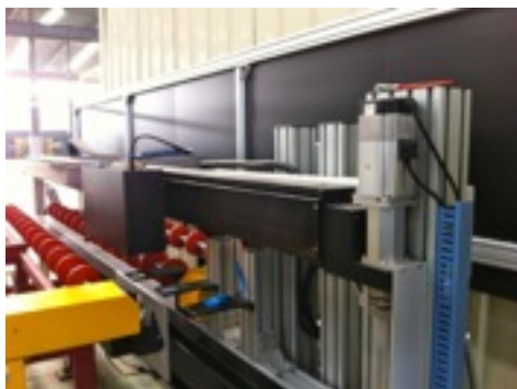
Left: 3 channel configuration (8 degree film- and glass-side reflectance, transmission) measurement system Right: Oblique angle (60 degrees) glass-side reflectance measurement system
